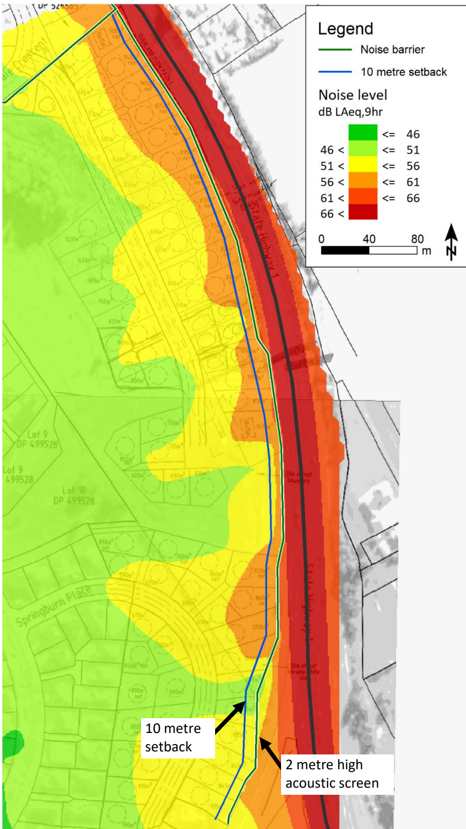
Figure A2 Predicted free field future traffic noise levels, L_{Aeq}(9 \text{ hour})
